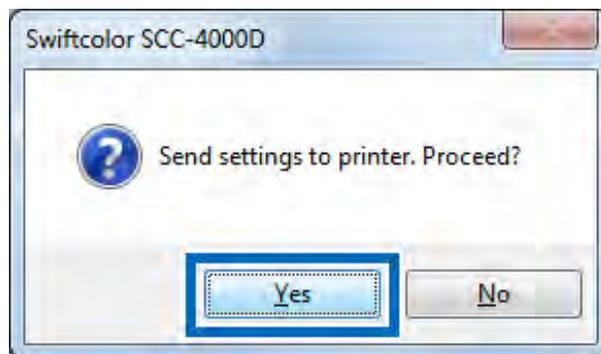
The adjustment value is transmitted to the printer to adjust the head positions.
