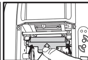
Place dust arrester back to the printer
